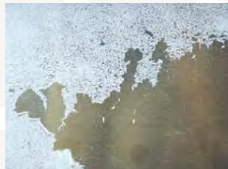
Img. 3.9.3. Insufficient wet out of the substrate
