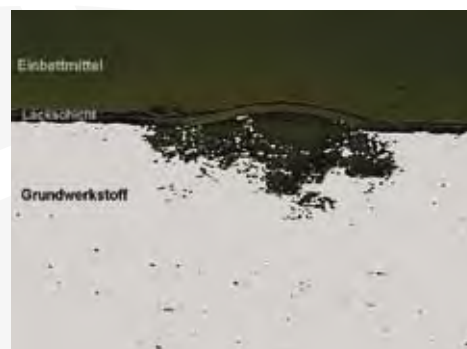
Img. 1.1.6. Comprised pretreatment-crystals (salts, chlorides)
