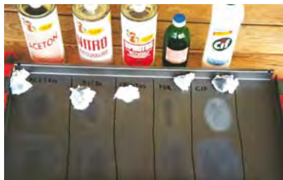
Img. 7.2.1. Greying caused by cleaning compounds
