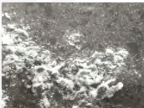
Img. 5.1.5. Mortar residues on the powder coat layer (microscope view)
