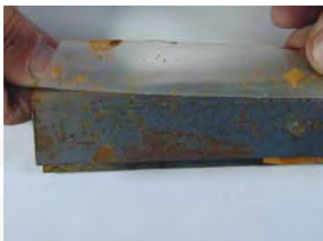
Img. 5.3.5. Infiltration caused by an insufficient pretreatment
