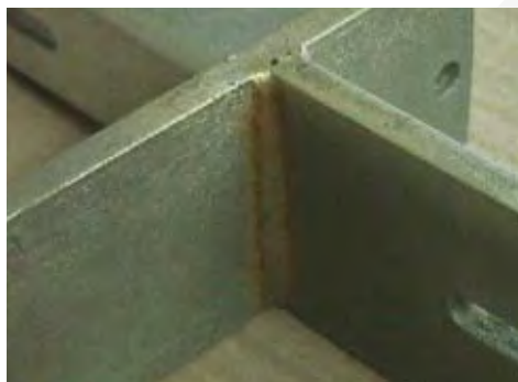
Img. 3.9.1. Insufficient wet out caused by corrosion
