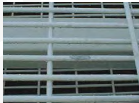
Img. 3.5.6. Uneven surface caused by poor zinc coating
