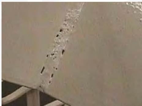
Img. 3.9.2. Insufficient wet out caused by oilcoat
