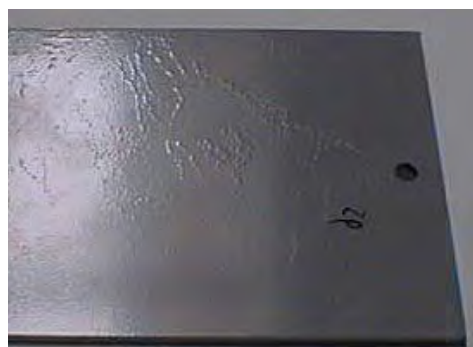
Img. 1.2.7. Poor purging, radiated, KTL-grounded
