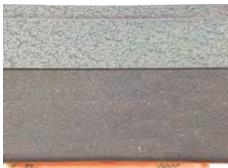
Img. 7.3.4. Effect-deviations caused by reclaim
