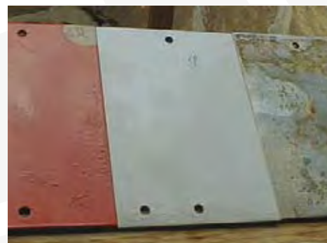
Img. 1.2.9. Poor purging, radiated, KTL-grounded and powder coated - comparison
