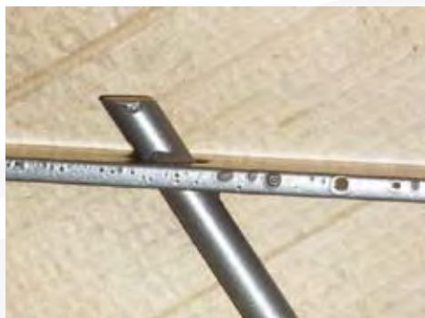
Img. 3.6.2. Bubbles caused by corrosion after pretreatment
