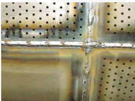
Img. 1.2.11. Oilcoal caused by welding work
