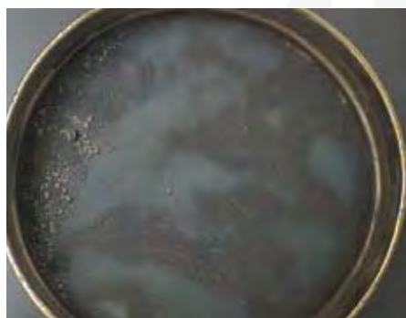
Img. 3.1.1. Filter residues cause powder spitters
