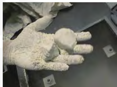
Img. 2.5.1. Powder lumping in the box
