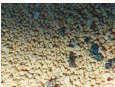
Img. 6.1.5. Dust in the reclaim powder (enlarged)
