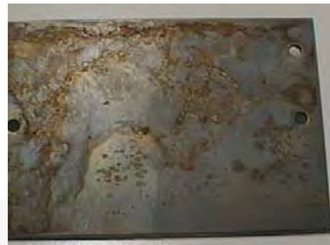
Img. 1.2.6. Poor purging, afterwards stored wet
