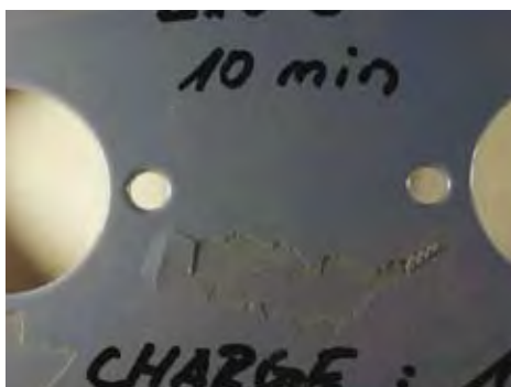
Img. 5.3.2. No adhesion of the top coat caused by directed heated gas oven
