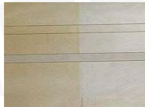
Img. 4.4.3. Yellowing in the interior caused by UV-light
