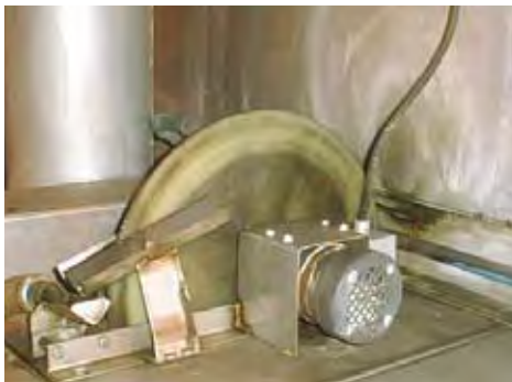
Img. 1.2.2. Primitive alternative of an oil separator
