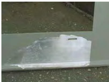
Img. 1.1.2. Poor (no) chromating
