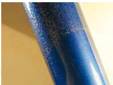
Img. 6.1.2. Contamination from poor equipment cleaning
