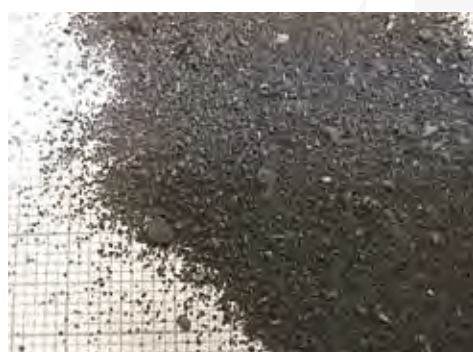
Img. 6.1.4. Dust in the filter residue
