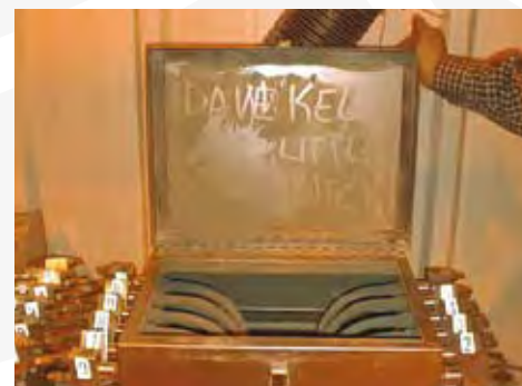
Img. 2.1.2. Poor fluidization - too much powder
