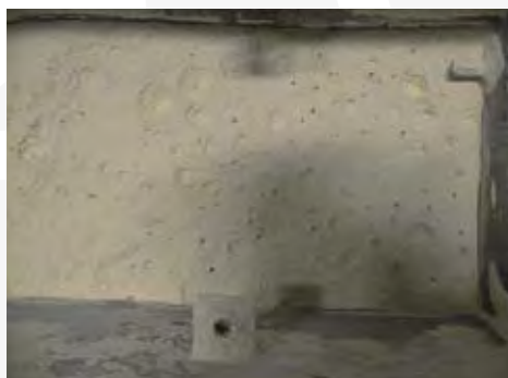
Img. 2.1.2. Poor fluidization
