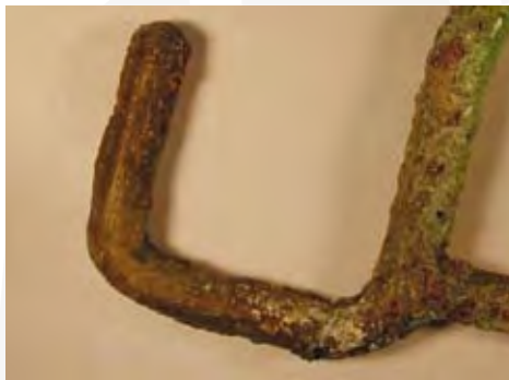
Img. 2.3.2. No earthing at multi coated hooks
