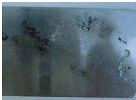
Img. 1.2.1 Fat-arrears after pretreatment
