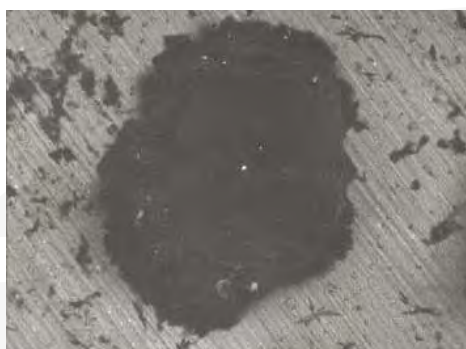
Img. 1.1.5. Residues on aluminum after pretreatment
